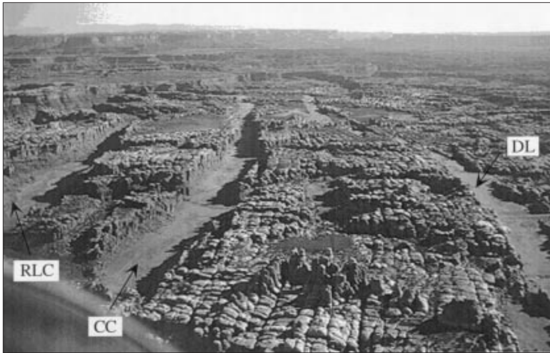
Figure 4. Oblique aerial photograph showing representative grabens and prefaulting jointed rock mass. Rectangular blocks in center of photograph are bounded by prominent joint sets, one trending northeast and the other trending northwest. View to north. DL—Deviils Lane graben (width, ~200 m); CC—Cyclone Canyon; RLC—Red Lake Canyon. Photograph by J. M. Moore.
